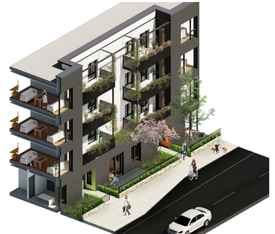
3D DRAWING SHOWING BLOCK F INTERFACE WITH STREET PRIVACY ZONE BETWEEN OWN DOOR GROUND FLOOR UNITS AND STREET
